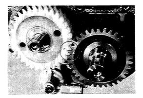
B. Remove the hexagon socket head cap screws from the cylinder block using a 6-mm hexagon wrench; extract the balance shaft and balance shaft gear toward the front of the cylinder block taking care to avoid damaging the bearing journals.
