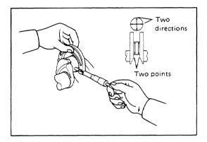
Allowable elliptical or tapered Limit: 0.0008 inches (0.02 mm)
