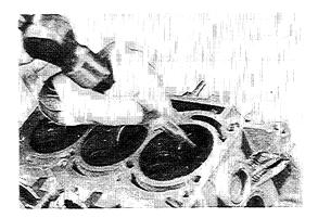
3. Place a clip on the new valve guide and drive it in from the opposite side of the combustion chamber with the valve guide installer.
