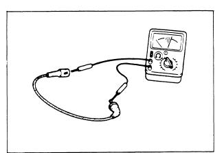
Specified resistance: Allowable limit: 16K Ohm/m 25K Ohm/m
