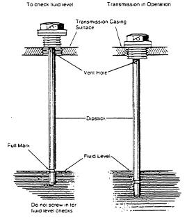
To check the fluid level, just insert the dipstick. Do not screw in. Retighten the hex screw with the dipstick after the fluid level check. Do not omit the O-ring seal.
