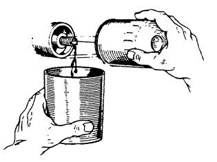
NOTE: Generic filters are not recommended, as the material standards or diameters of important items on generic parts might be entirely different from genuine parts. Immediately after an oil filter change and oil fill, run the engine to ensure that the oil pressure is normal and that there are no oil leaks around the new oil filter.
