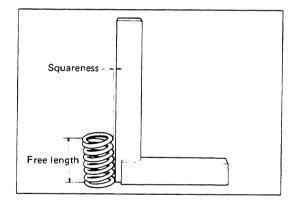
4. Using a spring tester, measure each spring's tension at the specified installed length. Replace the springs if they prove to be weakened.
