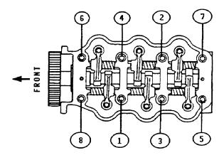
W 26G HEAD BOLT TIGHTENING SEQUENCE
