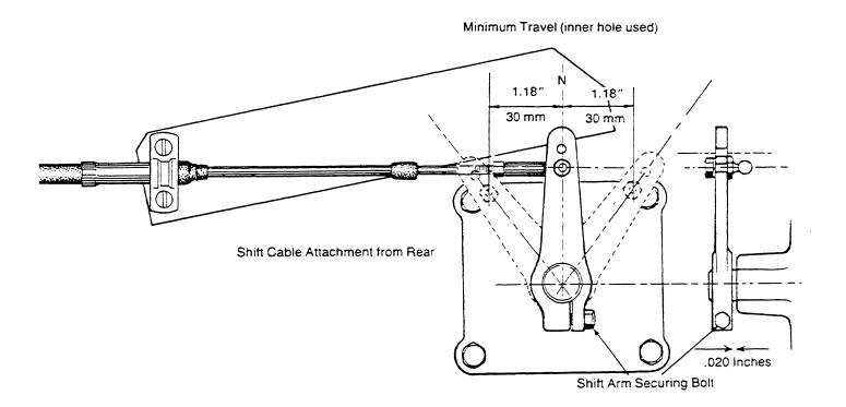
The position of the cover plate underneath the actuating lever is factory-adjusted to ensure equal lever travel from neutral to position A or B.
