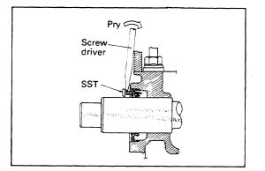
B. Screw the oil seal remover [SST] # 09233-87701-004 into the hole punched in step A.
