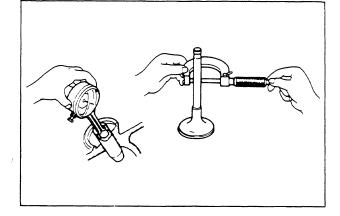
Measuring Method #2: Check each valve's deflection with a mounted dial indicator by moving the valve stem from side to side.
