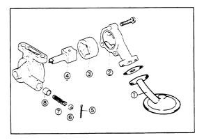
4. Measure the rotor shaft's clearance. If it has worn beyond the allowable limit, replace the rotor and the rotor housing.
