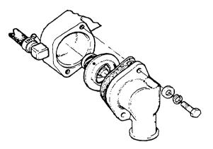
To test the thermostat, immerse it in water and gradually heat the water. The thermostat should start to open when the water temperature reaches 176 to 183° F (80 - 84° C). The thermostat should open by more than 0.31 inches (8 mm) when the water temperature reaches 203° F (95° C).
