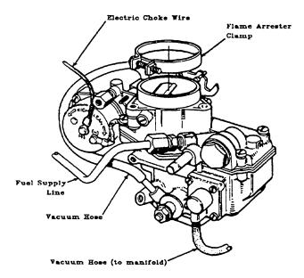
Carburetor with flame arrester removed.
