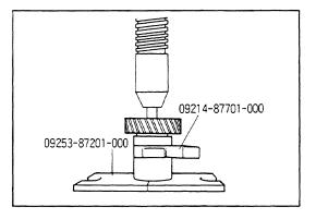
4. Replace the shaft's gear after the shaft has been refinished. Use special service tools # 09253-87201, 09506-87303, and 09214-87701.
