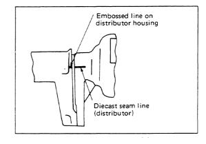
4. Temporarily tighten the distributor retaining bolt.
