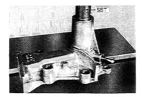
2. Using the same special service tools as in step #1, press off the water pump's bearing and seal set.
