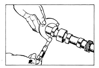
4. Measure the camshaft journal-to-cylinder head journal clearance. Replace the part that exhibits the most wear.
