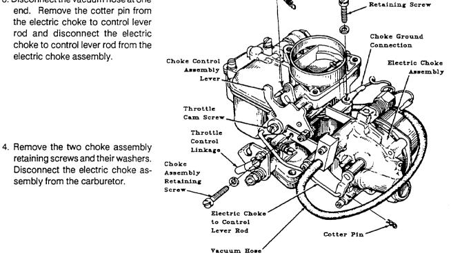
5. Remove the four cover screws and their washers. Lift the carburetor's top cover straight up and away from the carburetor's base. Take off the four screws holding the accellerator housing cover to the side of the carburetor body. Remove the cover, accellerator diaphram and spring. Inspect the diaphram and replace it if cracked or pourous.
