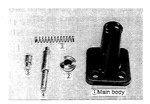
3. Place the small bar (5) into the piston pin. Then press the piston pin into position using a press.
