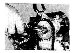
9. Install the balance shaft's gear cover.
