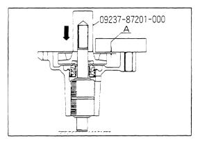
Press the water pump assembly into the water pump's pulley seat. Make sure that dimension H is maintained between 3.78 to 3.80 inches (96 - 97 mm)
