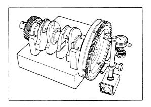
C. Heat the new ring gear to 250 - 300° C (480 - 570° F) on a hot plate or in an oven. Before slipping it onto the flywheel, make sure that the chamfered side of the ring gear is directed toward the engine.
