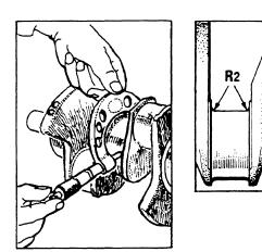
5. Measure the crankshaft's runout.
