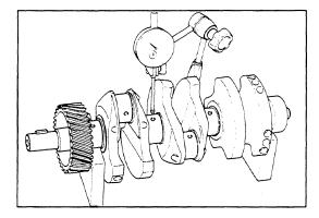
6. Measure the crankshaft for bend by placing a dial gauge at the center bearing journal and turning the crankshaft, as shown in the illustration to the right.
