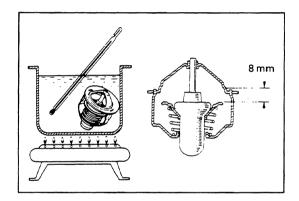
3. Replace the thermostat if the valve remains open at normal temperatures or if the valve is lose when the valve is fully closed.
