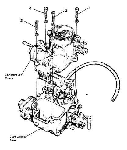
15. Reconnect the electric choke assembly to the carburetor and replace the two choke assembly retaining screws and their washers. Reattach the electric choke to control lever rod to the electric choke assembly and insert the cotter pin. Reattach the vacuum hose.
