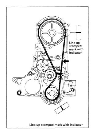
Rotate the crankshaft two complete turns in the normal direction of rotation until the No. 1 piston returns to Top Dead Center (TDC). Check that the timing belt pulleys again are properly aligned with their respective indicators, as indicated in step 5.
