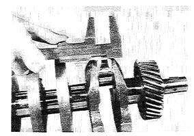
5. Measure the connecting rod width.
