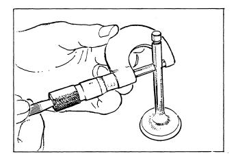
Check of each valve's head stock thickness. Replace the valve if it is beyond the allowable limit.
