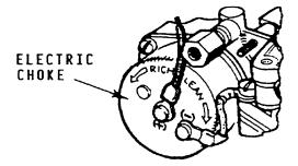
The choke housing will normally get hot during engine operation.
