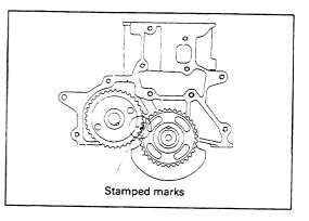
8. Install the oil pump's drive chain.
